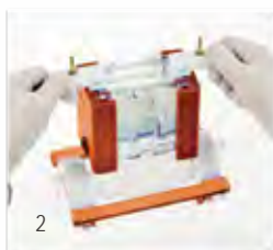
2 Transfer to casting base and tighten cams.
